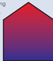
Fig. 13: Thermal layers in a heated, high ceilinged room*.
